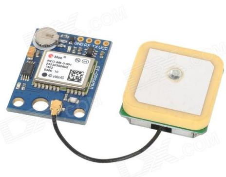
Figura 7: Módulo GPS GY-GPS6MV1.
