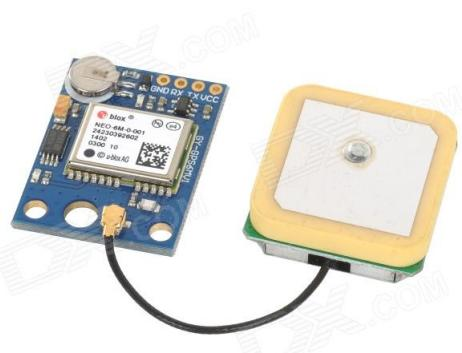
Figura 7: Módulo GPS GY-GPS6MV1.
